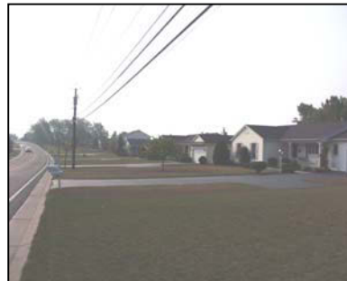
Frontage development can create access management problems if individual driveways are permitted for each home (left). Frontage development is also inefficient -- once the frontage is all developed (top right), developing the interior lands (bottom right) is very difficult because proposed new homes are likely to be in the “backyards” of the ones already built along the road frontage.
